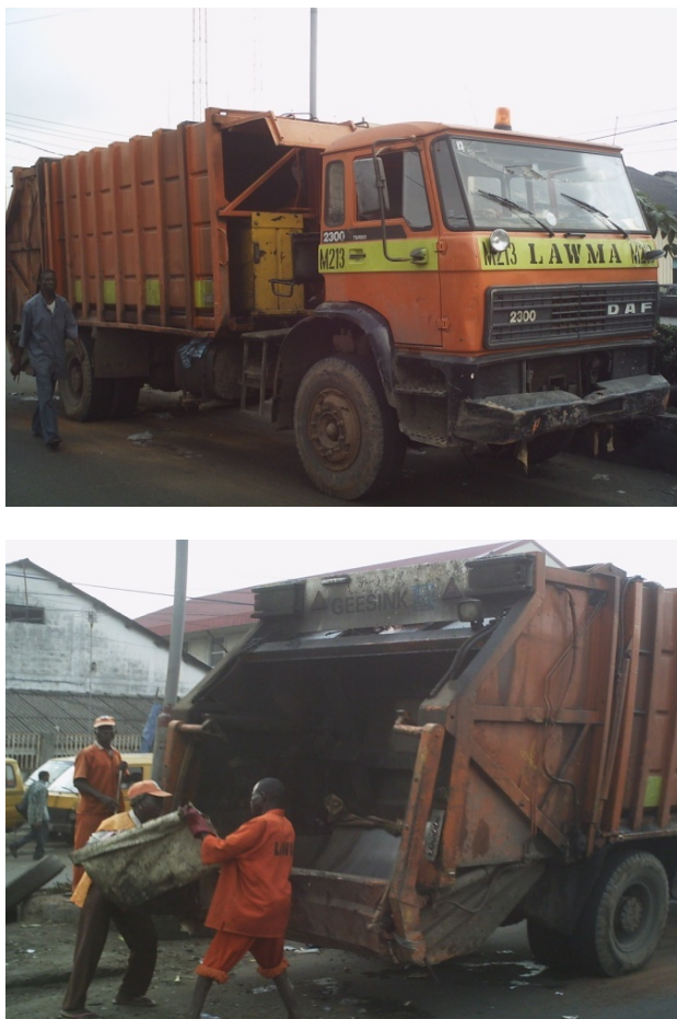
Fig. 1. Solid waste collection vehicles with hydraulic ram
