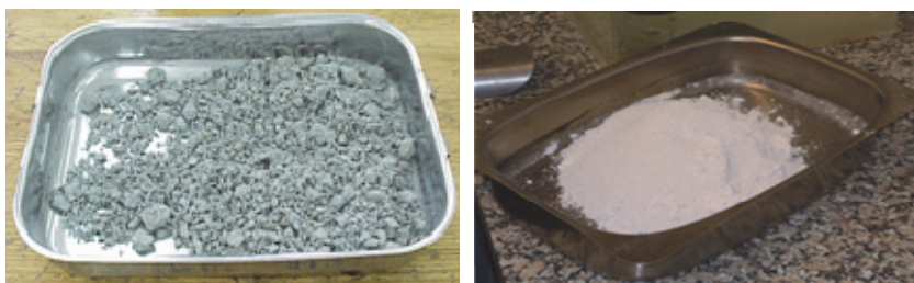
Fig. 1. Appearance of the sludges before (left) and after calcination (right)
