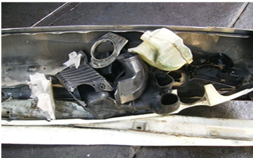
Fig. 5. Recovered plastics from a commercial vehicle
